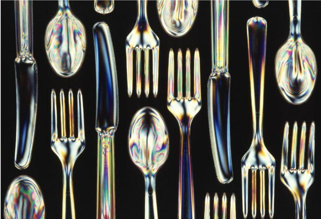
**A picture of plastic utensils created using photoelasticity**
