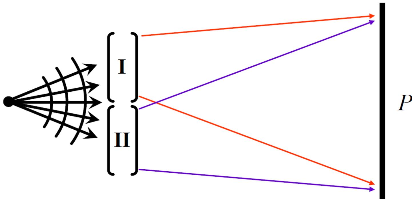
$$\begin{cases} \varphi_1(P) = \varphi_0 + \frac{2\pi}{\lambda} (SIP) \\ \varphi_2(P) = \varphi_0 + \frac{2\pi}{\lambda} (SIIP) \end{cases} \quad \longrightarrow \quad \Delta\varphi(P) = \frac{2\pi}{\lambda} [(SIP) - (SIIP)]$$
